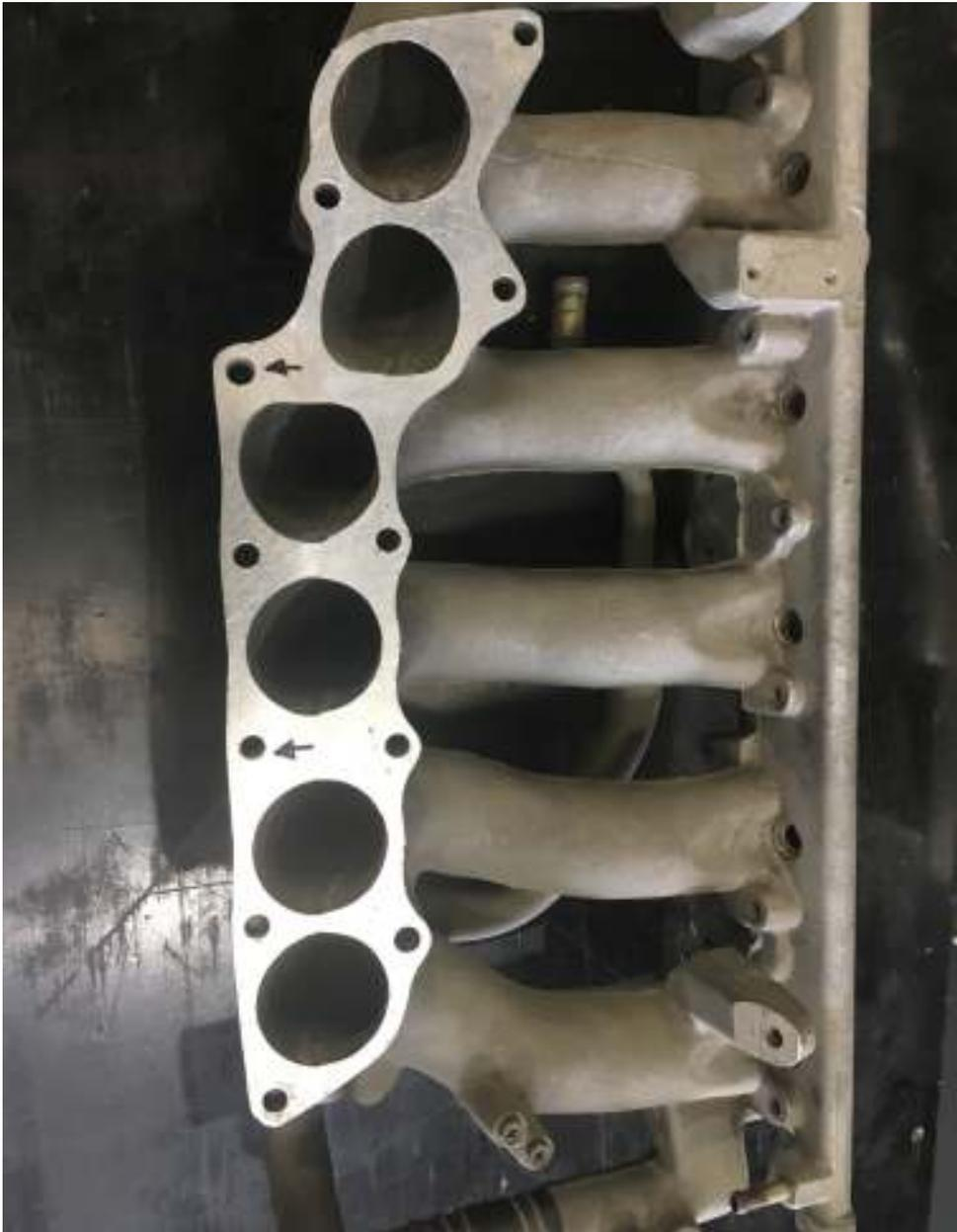
4. Once drilled, clean out all alloy swarth and clean off any old gasket paper or residue that can be found on the top surface .
