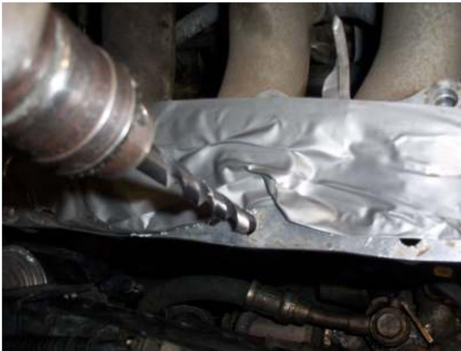
3. Drill out x2 threaded holes with a 8.5 – 9mm drill bit. **THE HOLES MARKED WITH AN ARROW BELOW**
