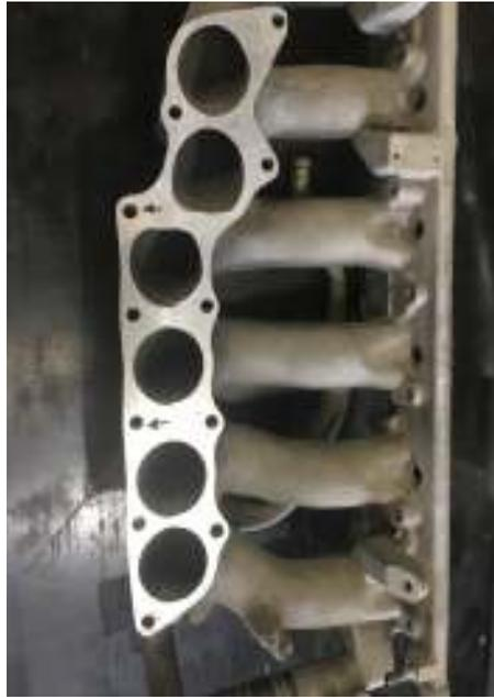
4. Once drilled clean out all alloy swarth and clean off any old gasket paper or residue .
